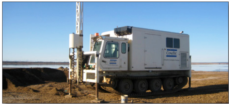
Figure 3. Tracked CPT rig (photo courtesy of Conetec)
