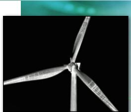
Ground-based wind turbine inspection technology can detect defects and anomalies in turbine blades while operating.
