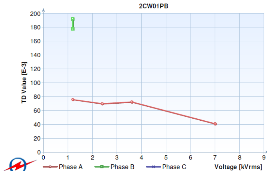
Figure 9-6 Tan \delta test with negative delta tan \delta identified bad splice
