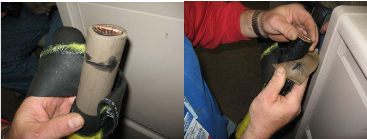
Figure 7-6 New splice of a 15-kV cable operated at 13.8-kV that failed at the 12-kV \tan \delta step prior to the 16-kV withstand test
