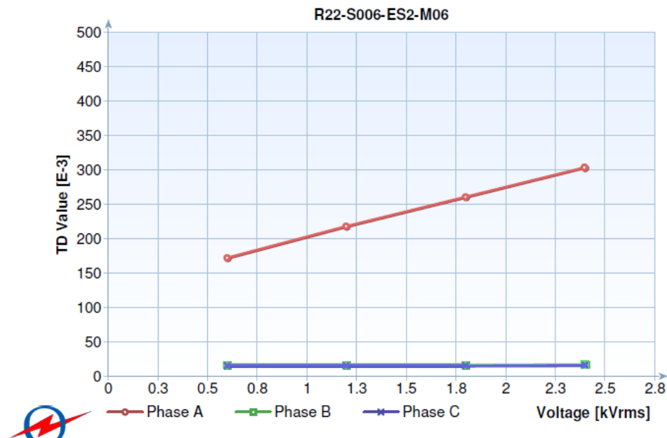
Figure 9-5 “Action required” delta tan \delta test results
