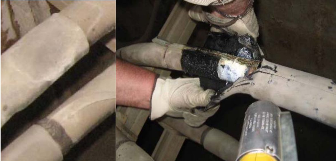
Figure 7-5 Splice with a poor heat shrink being opened and exposing the degraded zinc metallic insulation shield
