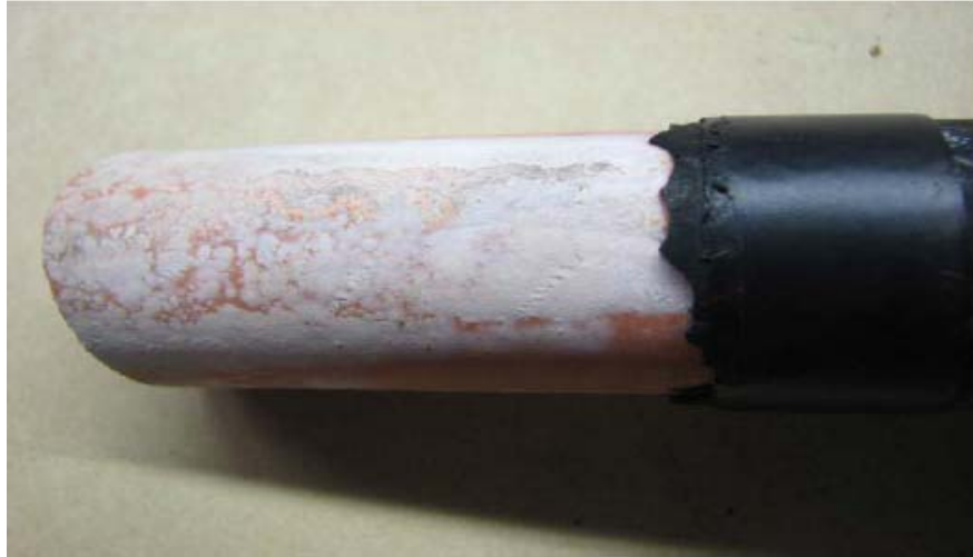
Figure 6-4 The white substance in the figure is the partial-discharge-affected surface of the EPR insulation.
