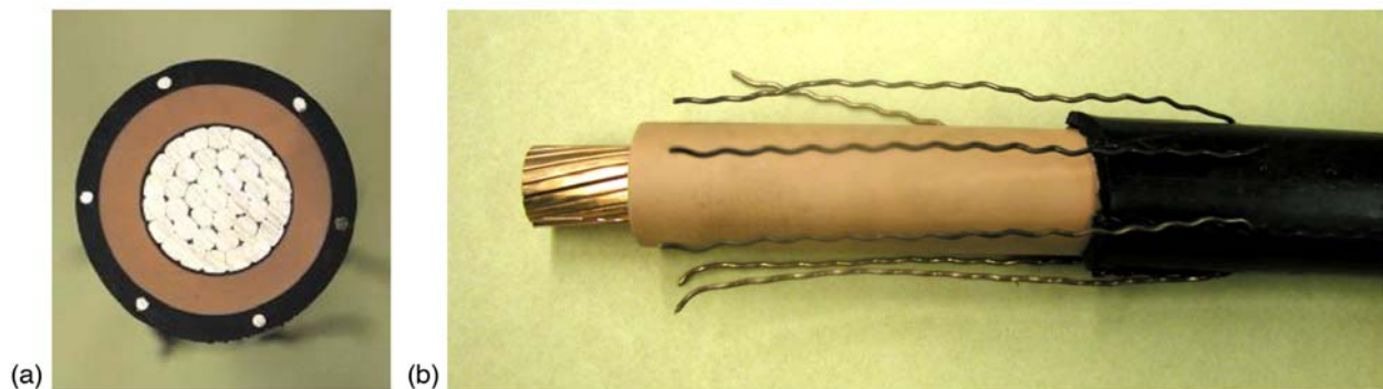
Figure 6-1 Construction of pink EPR compact design cable [a] transverse view, [b] lengthwise view
