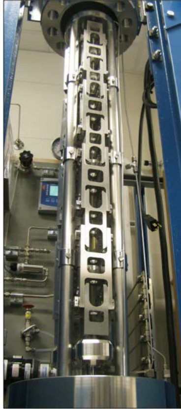
Figure 4-2 Early version of the PNNL 3-string design capable of holding 24 specimens
