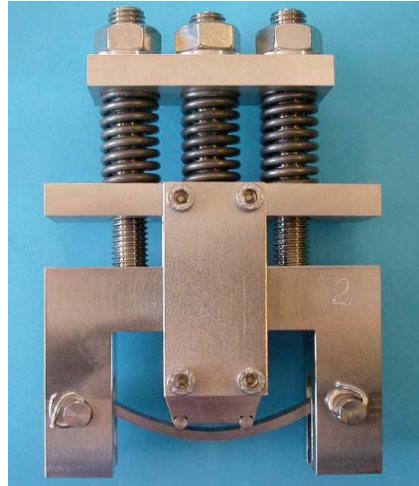
Figure 3-2 4-point bend devised by AREVA [12]
