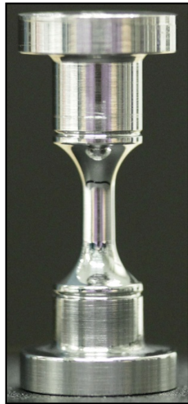
Figure 3-4 PNNL 1.2" tall SCC tensile initiation specimen
