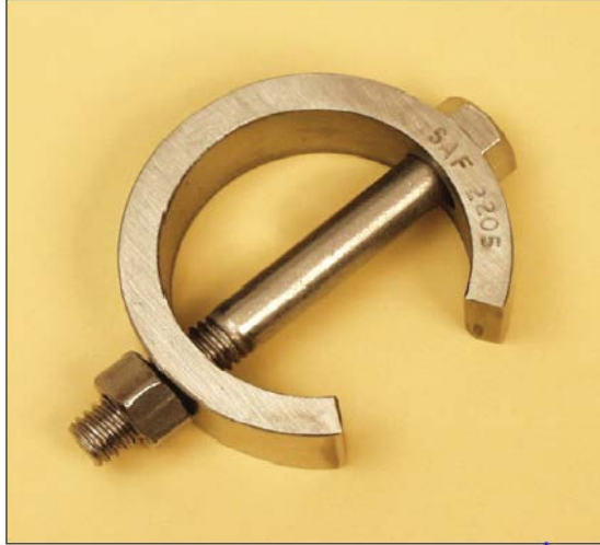
Figure 3-3 C-ring specimen from ASTM G38-01 (2013) [13]
