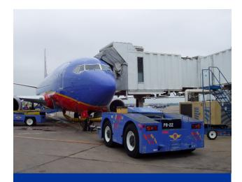
Around the world, airports and airlines face pressure to meet increasingly stringent air quality standards and reduce costs. In response, many are replacing internal combustion ground support equipment with electric GSE that offers comparable functionality, reduces emissions, and lowers operating costs. Retrofit kits and new electric equipment are available.
