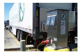
TSE can also power electric-standby transport refrigeration units and generators, or "gen-sets."
