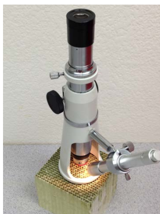
Figure 3-6 Example of Microscope Used to Document Catalyst Cell Dimensions
