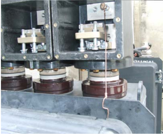
Test 2012-2: A \Phi to case; 0.53 cycles
