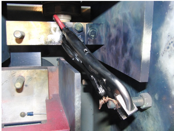
Test ID 18: AΦ to Front Bolt- Vise Grip - 1.5 cycles
