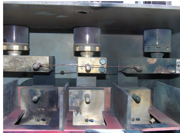
Test ID 44: AΦ-BΦ-CΦ 20AWG without Barrier - 0.28 cycles
