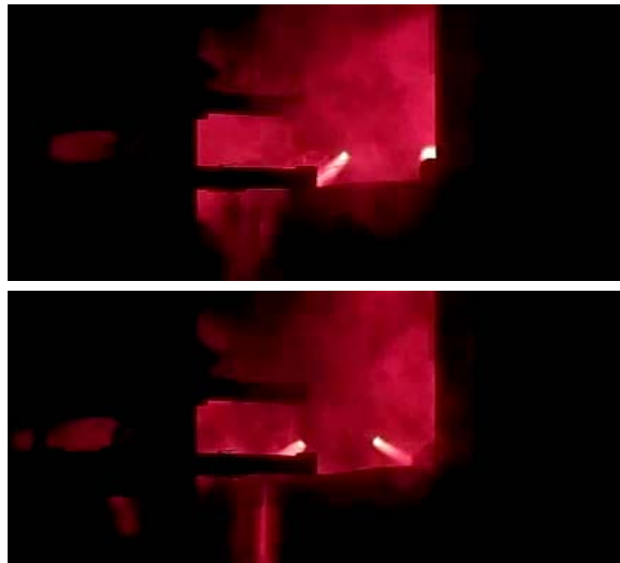
Figure 2-16 Examples of arc paths with the end barrier in the 2009 tests in a network protector
