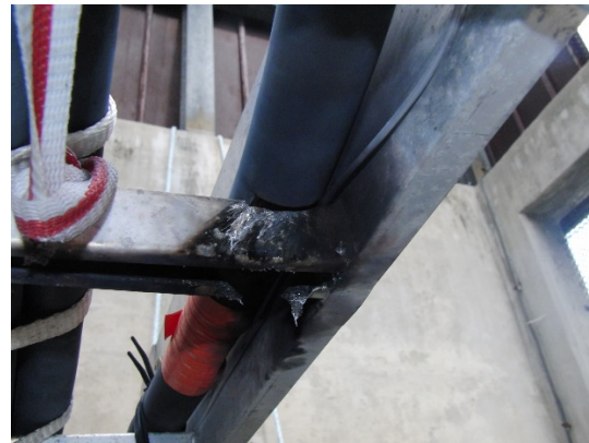
Figure 3-2 (continued) Cable tray arc initiation points, arc durations, and post-test damage
