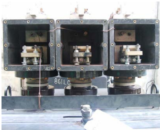
Test 2012-7: Three-phase to case; 0.45 cycles
