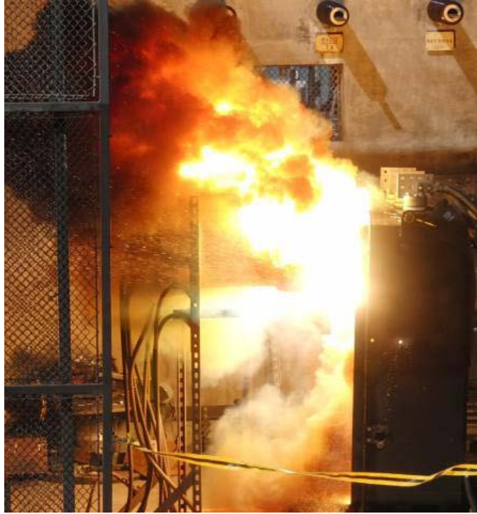
Figure 1-1 Example 480-V network protector event [EPRI 1020210, 2009]
