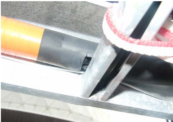
Figure 3-2 (continued) Cable tray arc initiation points, arc durations, and post-test damage
