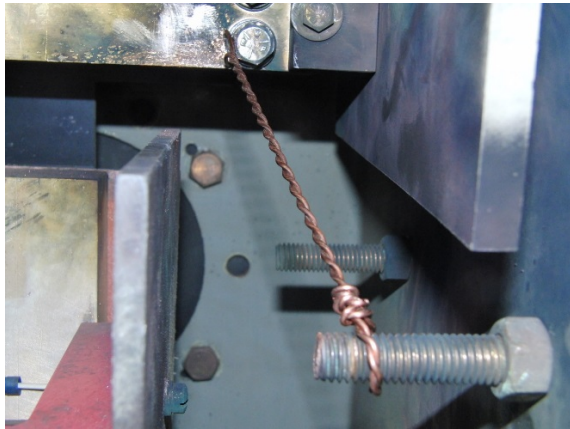
Test ID 17: AΦ to Front Bolt- 2-14 AWG - 0.51 cycles
