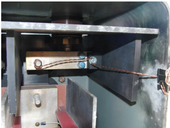
Test 15: AΦ to Case - 2-#14 - 0.35 cycles
