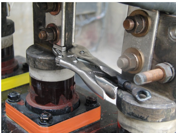
Test ID 48: AΦ-BΦ vise grip; 2.65 cycles
