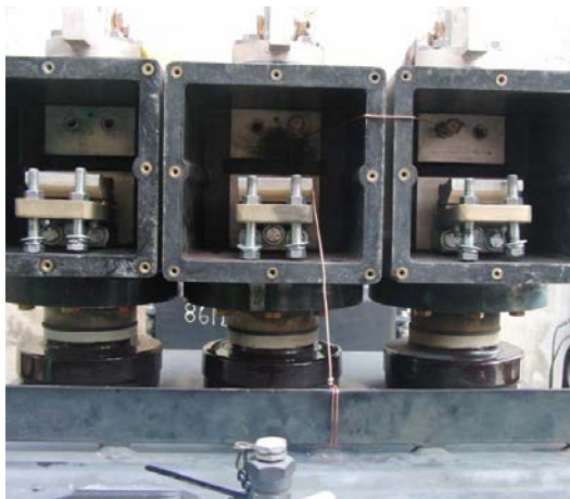
Test 2012-5: B \Phi to A \Phi to case; 0.67 cycles
