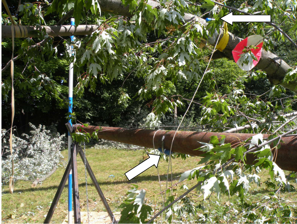
Figure 3-6 Branch specimen and test jig following a drop test.
