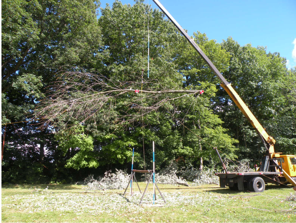
Figure 3-5 A defoliated branch specimen in free fall above the target.
