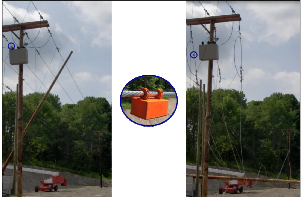
Figure 12-7 Position of the conductor sensor before and after the test
