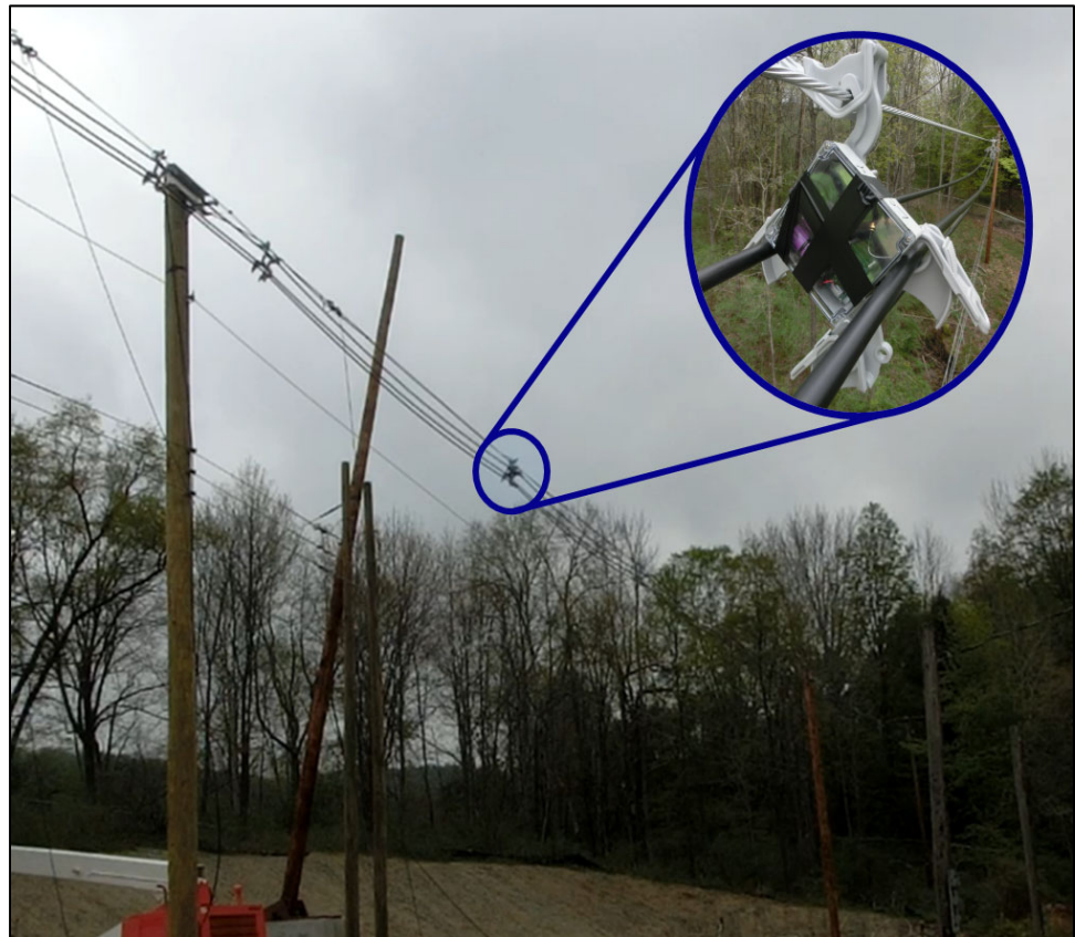
Figure 12-3 Spacer cable testing at Lenox laboratory. Note the sensor is attached to spacer during this full-scale test.
