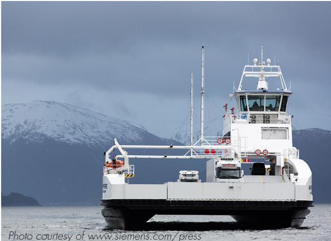
The *Ampere*, the world's first electric battery powered car and passenger ferry, entered operation with Norled in January 2015 in Norway. The nearly 250-foot long electric catamaran was designed as part of a competition launched by Norway's Ministry of Transport and Communications in 2011 to develop an environmentally friendly ferry serving in the region. Norled, a shipping and ferry company in Norway, won the competition with their design.
