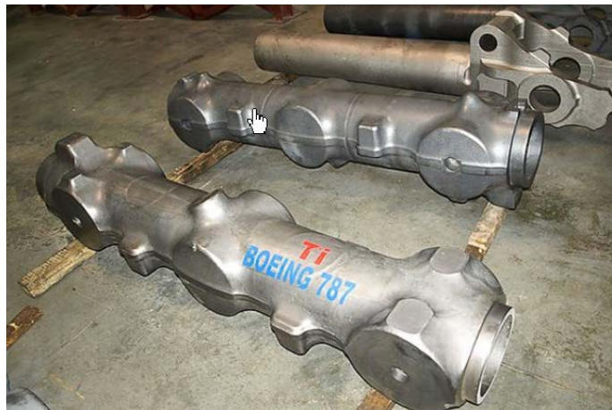
Figure 2-2 High strength titanium landing gear that has been forged
