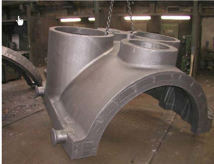
Figure 2-5 Application of HIP to large castings could be used to eliminate hours of repair and rework often applied to such structures
