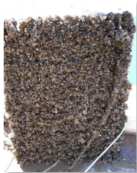
Figure 1 – A completely fouled metal grate shows the extent to which biofouling can affect submerged structures (Image from Skaja et al. 2014).
