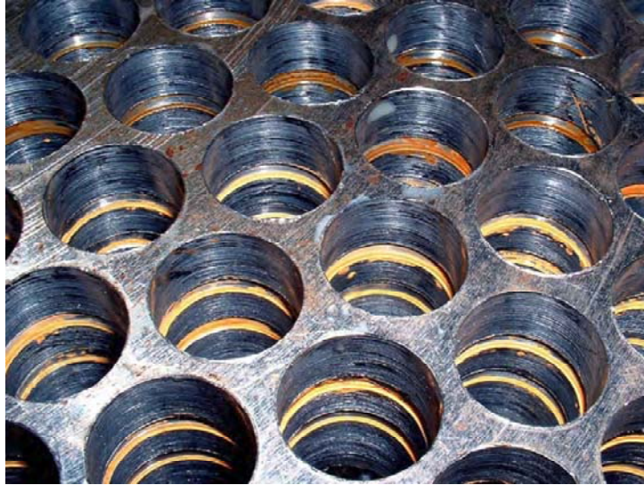
Figure 3-18 Example of TEMA Grooves in Tubesheet Holes
