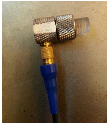
Figure 3-7 5-Mhz, 1/4-inch-diameter contact transducer shown with delay line attached
