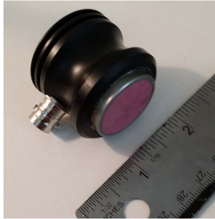
Figure 3-16 2.25-MHz, \frac{3}{4} -inch-diameter element contact transducer
