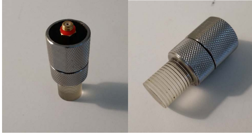
Figure 3-14 1.0-MHz, 1/2-inch-diameter single-element contact transducer with 1-inch delay line
