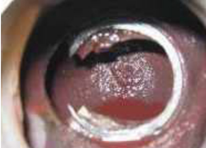
Figure 4-7 Liquid Droplet Impingement on High Pressure Coolant Injection Steam Line Drain Pot Valve Body and Internals [19]
