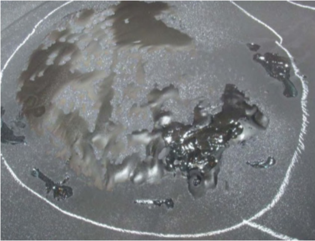
Figure 4-12 Main Steam End Cap Liquid Droplet Impingement [25]
