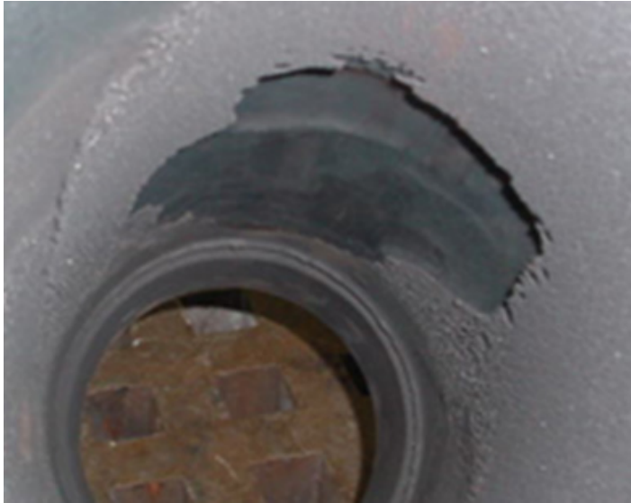
Figure 4-15 MSR Vent Line Liquid Droplet Impingement [3]
