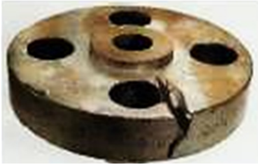
Figure 6-3 Pipe Flange – Steam Cutting Erosion [8]
