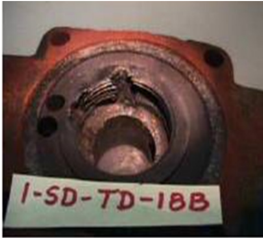
Figure 6-4 Steam Trap Body – Steam Cutting Erosion [8]
