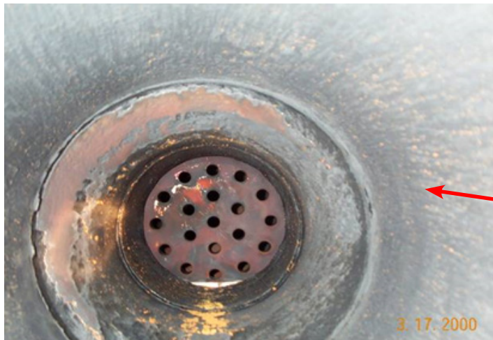
Figure 3-1 Reactor Feedwater Pump Minimum Flow Line to Condenser – Flashing Flow Erosion [2, 3, 11]
