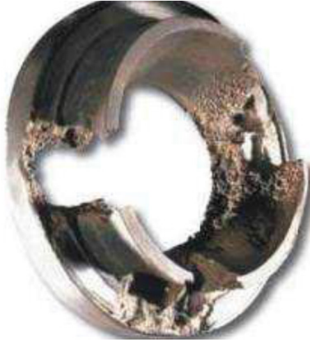
Figure 2-9 Control Valve Trim - Cavitation Erosion [8, 19]
