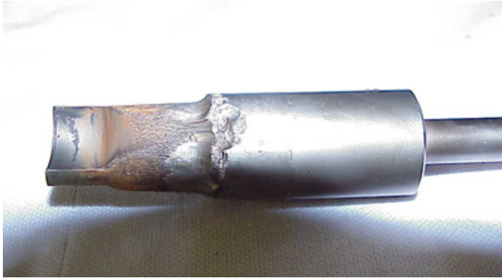
Figure 5-5 Steam Generator Blowdown Valve Internal – Solid Particle Erosion [2, 3, 8]
