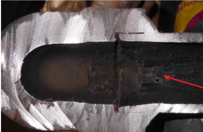
Figure 3-3 Reactor Feed Pump Turbine (RFPT) Main Steam Supply Drain Line – Flashing Flow Erosion [18]
