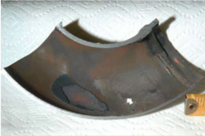
Figure 8-16 Steam Seal Leak in Elbow – Two Phase Flow Accelerated Corrosion [24]
