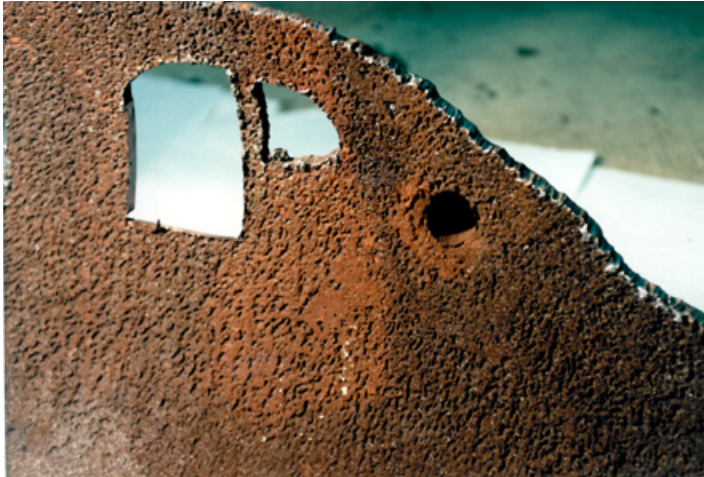
Figure 4-19 Low Pressure Extraction Steam Line Degradation from Liquid Droplet Impingement [26]
