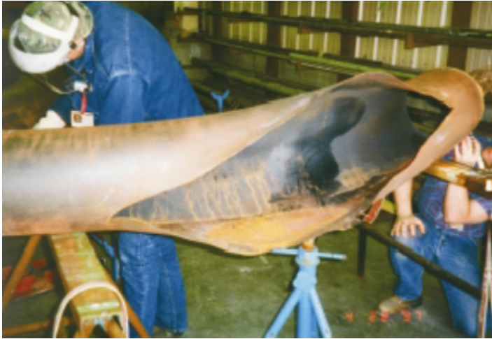
Figure 8-20 High Pressure Extraction Steam Bend Failure – Two Phase Flow Accelerated Corrosion [9]
