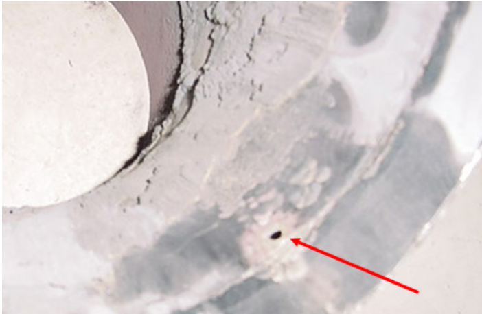
Figure 4-16 Extraction Steam Line Combinations of LDI and FAC [3]
