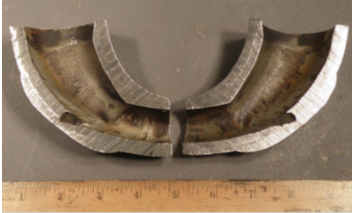
Figure 2-13 Steam Generator Blowdown - Cavitation/Liquid Droplet Impingement Erosion [21]
