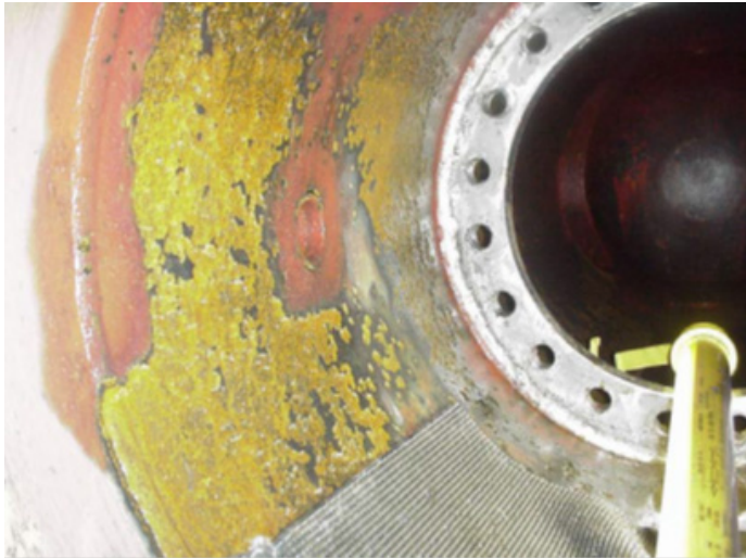
Figure 10-8 Degradation within Resin Trap [6]
