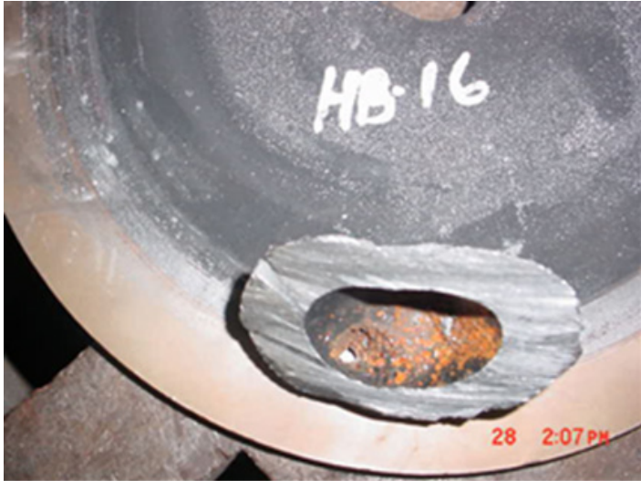
Figure 2-25 Condensate Pump Equalizer Line Downstream of Orifice – Cavitation Erosion [3]
