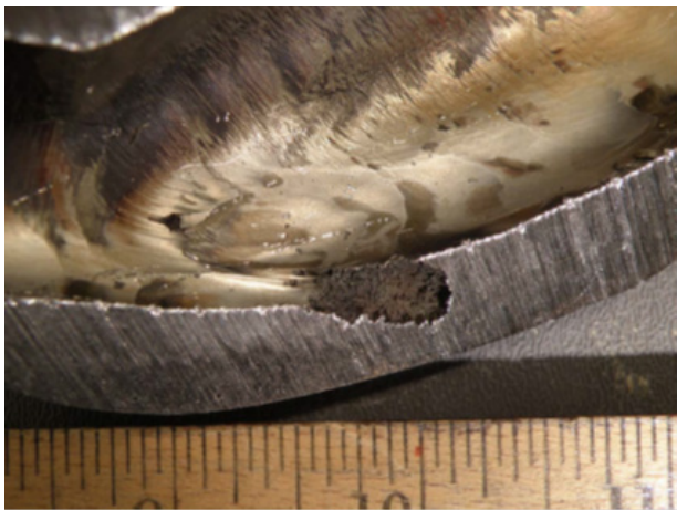
Figure 2-14 Steam Generator Blowdown – Close-Up of Degraded Surface - Cavitation/Liquid Droplet Impingement Erosion [21]
