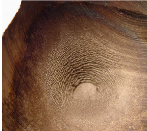
Figure 4-18 Feedwater Heater Vent Line P22 Socket Welded Elbow Downstream of an Orifice [3]
