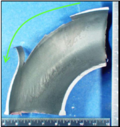
Figure 8-13 Reheat and Moisture Separator System Side View of Failed Elbow – Two Phase Flow Accelerated Corrosion [24]
