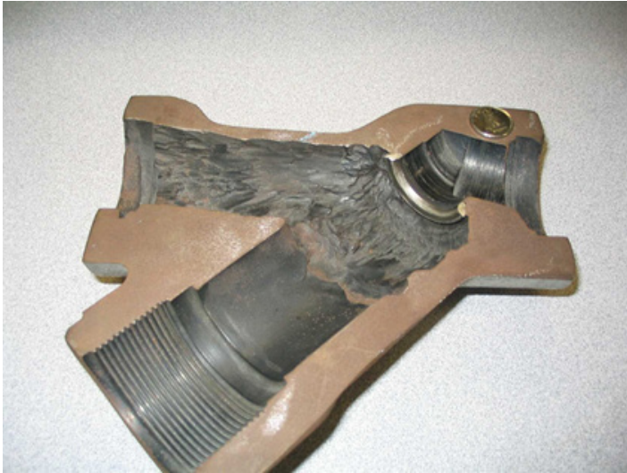
Figure 5-3 Boiler Blowdown Valve Body – Solid Particle Erosion [3, 19]
