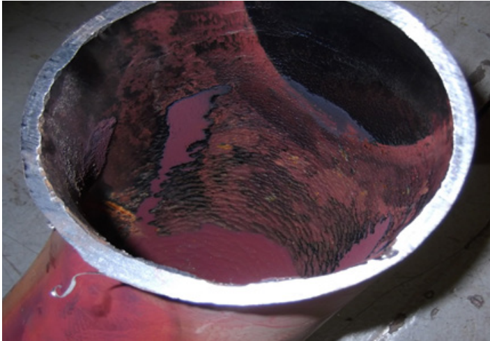
Figure 4-20 Miscellaneous Equipment Drain Header Elbow Degradation from Liquid Droplet Impingement (Photo Courtesy of TVA)
