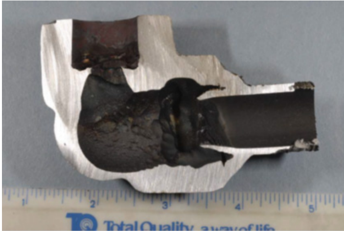
Figure 7-3 Socket Welded Connection Downstream of Normally Closed Valve – Single Phase Flow Accelerated Corrosion [13]
