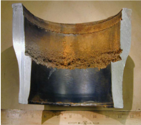
Figure 2-6 Reducer Constructed of P22 Material on 8" (20.3 cm) Feedwater Recirculation Line - Cavitation Erosion [3, 18]
