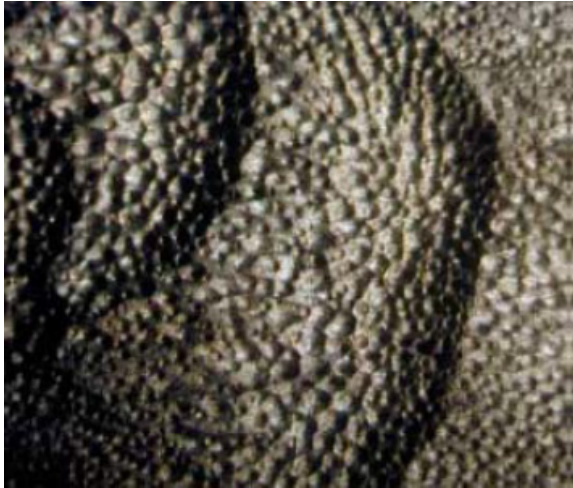
Figure 10-10 Low Temperature FAC Surface Degradation shows Rippled Surface [9, 27]
