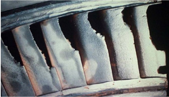
Figure 5-6 Turbine Blade Damage – Solid Particle Erosion [8]
