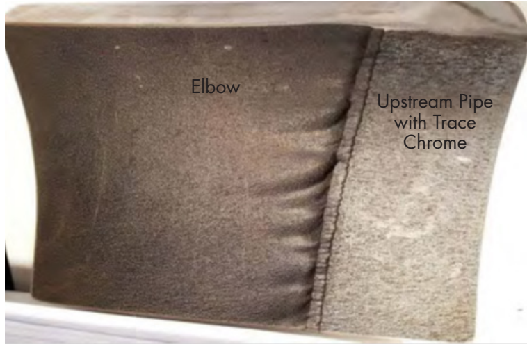
Figure 7-11 Carbon Steel Feedwater Elbow Downstream of Carbon Steel Pipe with Trace Chrome – Single Phase Flow Accelerated Corrosion [25]
