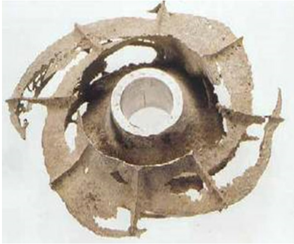
Figure 2-21 Pump Impellor – Cavitation Erosion [2, 8]
