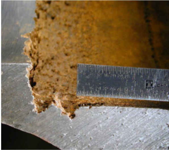
Figure 2-7 Close-Up View of Degraded Surface of P22 Fitting - Cavitation Erosion [3, 18]
