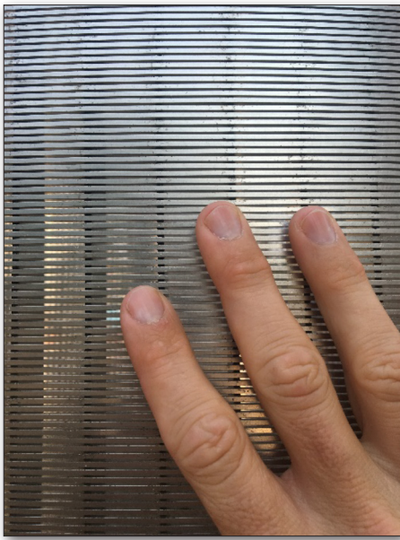
Figure 6. Wedge wire slot width of 0.75 mm at Cayuga Power Station [photo courtesy of ISI]
