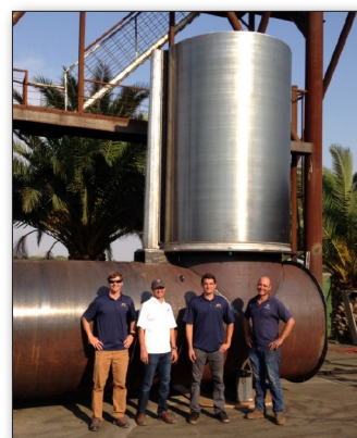
Figure 5. Cylindrical wedge wire half screen with external (and internal) cleaning brush [photo courtesy of ISI]
