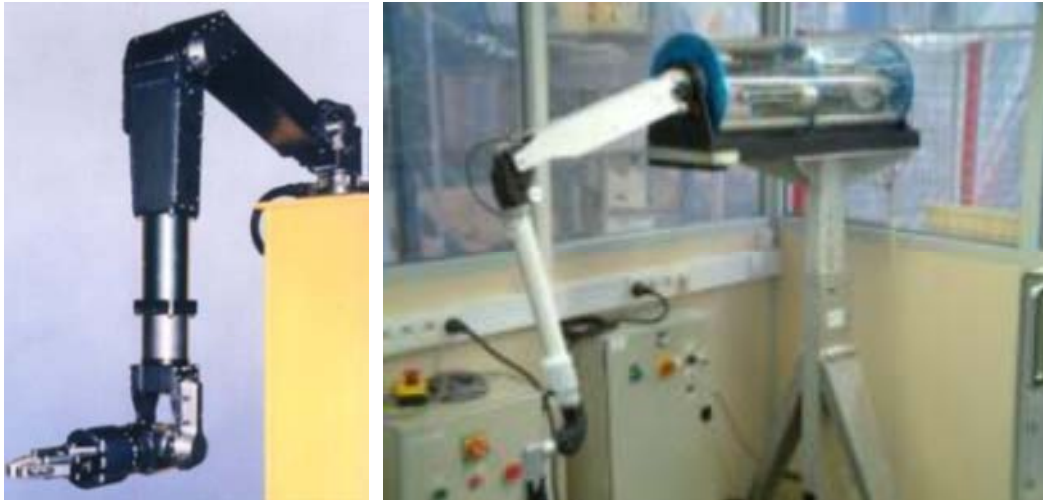
Figure 5-1 MAESTRO System Slave (a) and Master (b) Arms [27]
