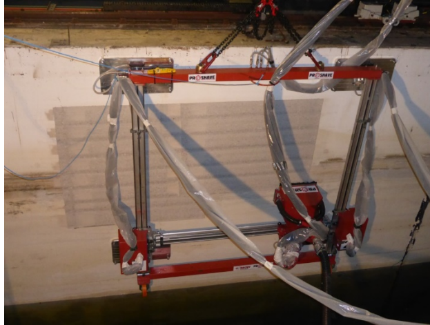
Figure 7-3 Remotely Wall Mounted Shaving System [43]
