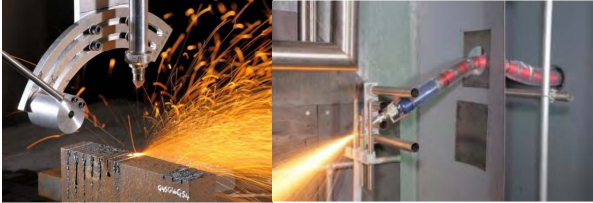
Figure 5-2 Gouge Cutting and 1.5m, 100mm Diameter Snake Arm [27]
