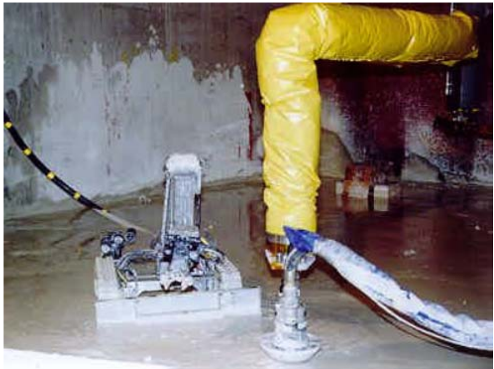
Figure 4-1 Houdini Remotely Operated Vehicle (left) with Confined Sluicing End-Effector Tool (right) [16]
