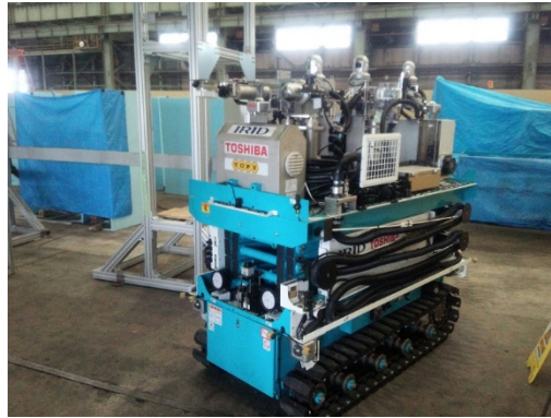
Figure 7-5 Dry Ice Decontamination Robot [47]
