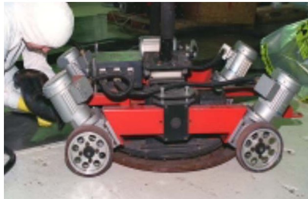
Figure 7-1 En-Vac Remote Wall Scabbler [16]
