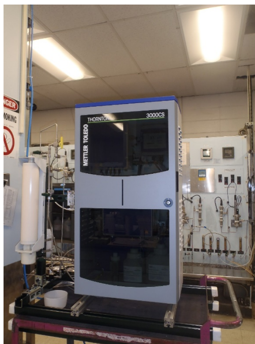
Figure 2-1 Chloride and sulfate analyzer setup in the Labadie chemistry lab
