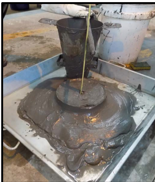
Figure 1-1 Slump testing results showing a flowable paste material
