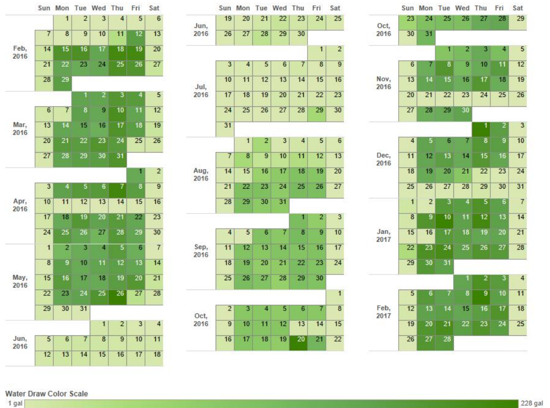
Figure 2-4 Calendar of test period, with color scale showing the range daily hot water used over 13 months
