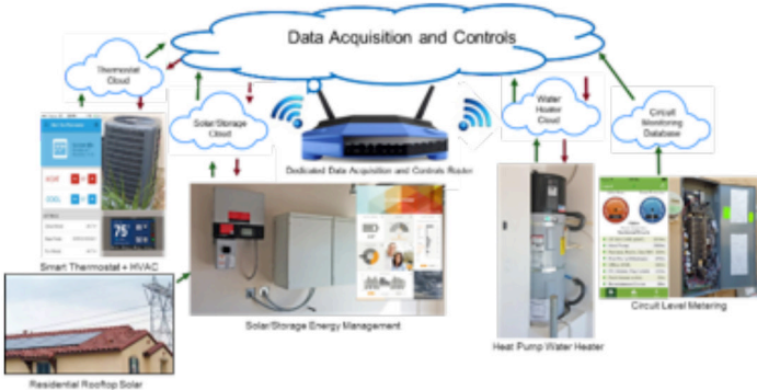
Figure 5 – Data Integration and Control Architecture
