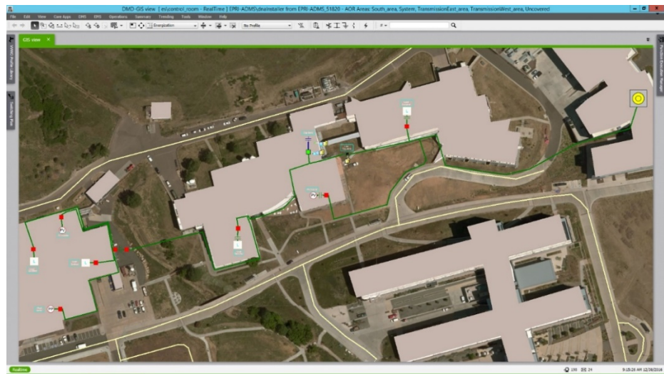
Figure 2-1 ADMS GIS view of a fictitious test feeder on a generic land base.
