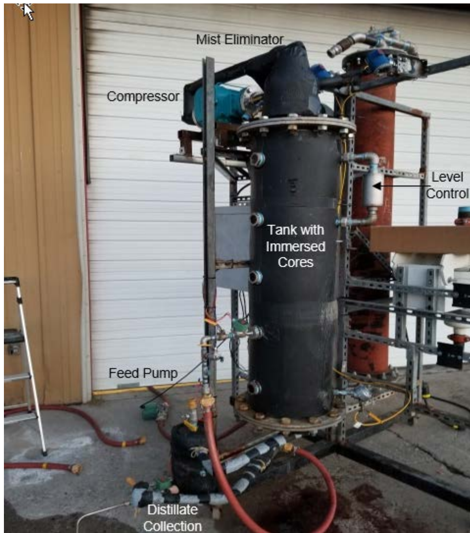
Figure 3-1 Lab-scale AVARA 0.2-GPM test unit
