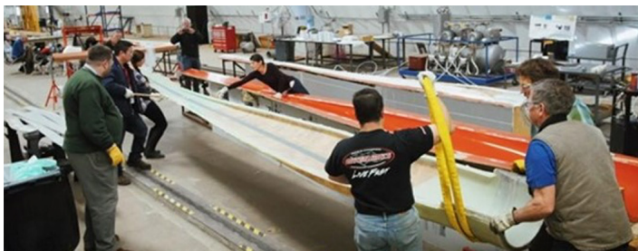
Figure 7 – Image of the NREL/IACMI thermoplastic wind turbine blade prototype (Source: Composites World)
