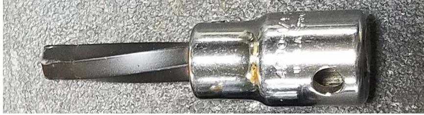
Figure 3-9 Distortion and permanent twisting of a hex key
