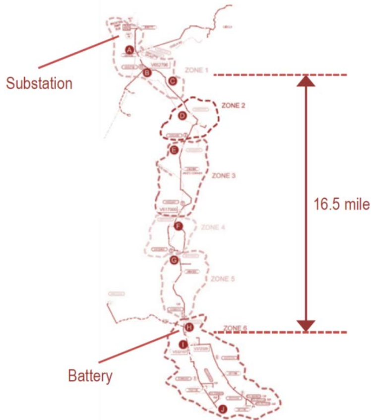
Figure 3-2 The Mazatzal Feeder, Substation, and Battery Unit Serving Punkin Center, AZ
