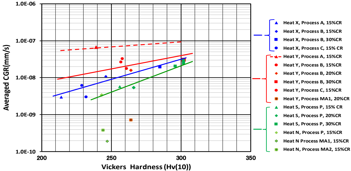
Figure 4-3 Relationship between CGR and Vickers hardness for Alloy 690 cold rolled to various thickness reduction levels [34]
