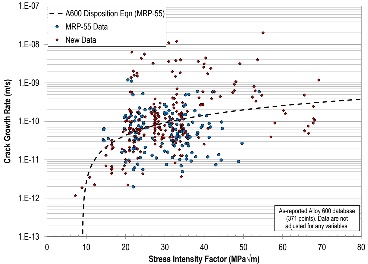
Figure 3-3 Screened Alloy 600 database: All data, unadjusted for temperature, dissolved hydrogen, cold work level, etc. Comparison is shown between MRP-55 data and newly compiled data.
