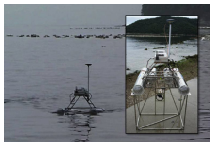
Figure 4 – Jellyfish Elimination Robotic Swarm or JEROS was constructed by a group at the Korean Advanced Institute of Science and Technology (Ackerman 2013)
