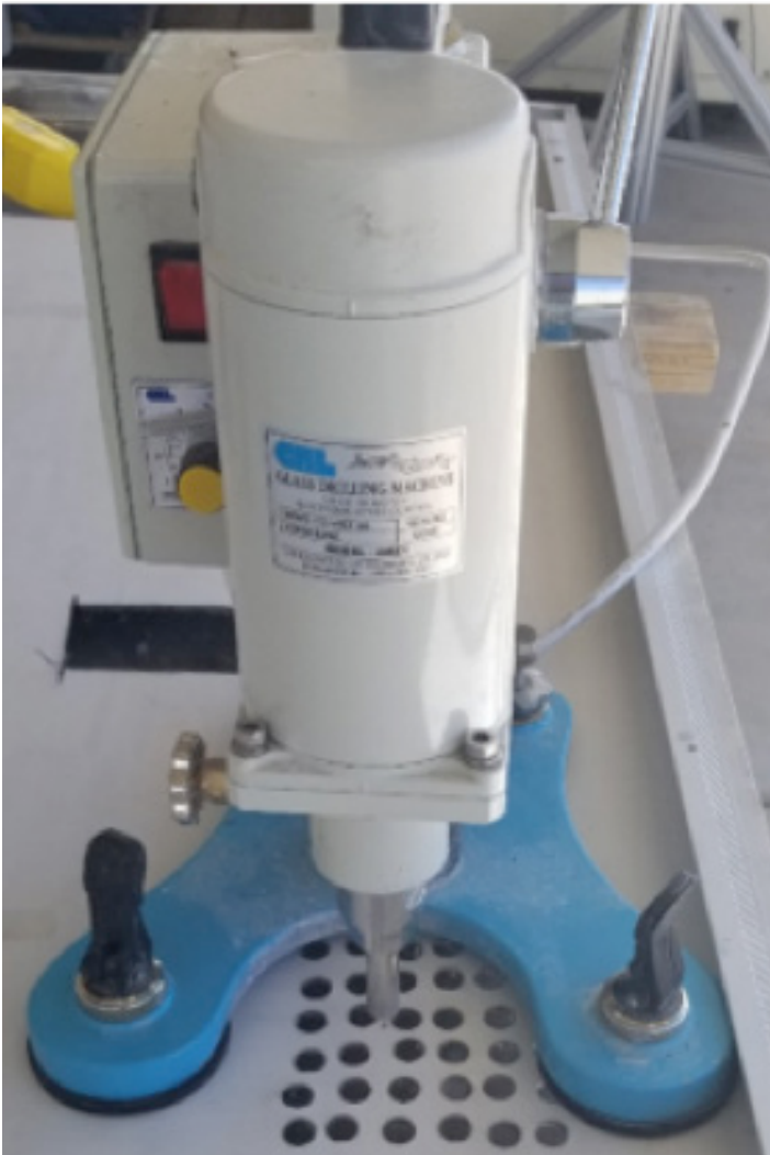
Figure 16 - Mechanical coring process setup (Photo Credit: ASU)
