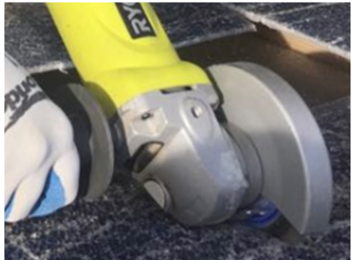
Figure 15 - Water-jet extraction module core samples (top); and strip-cutting sampling process (bottom) (Photo Credits: ASU)
