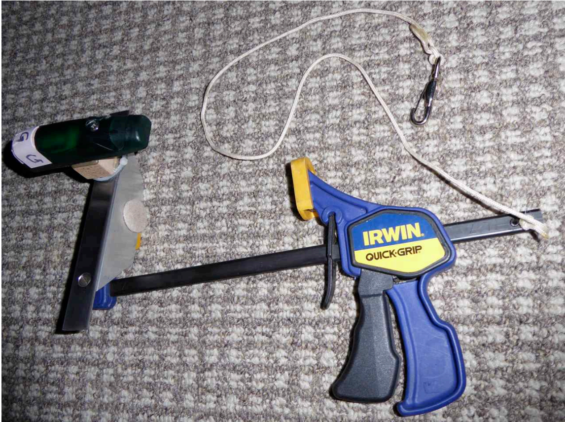
Figure 4-3 Workshop clamp modified to mount accelerometer to non-magnetic materials
