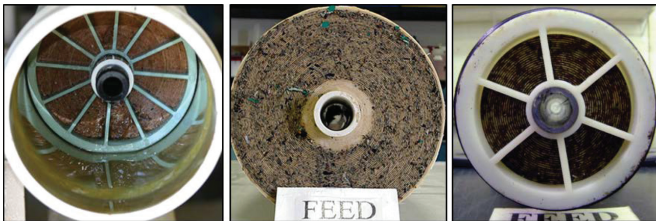
Figure 2 – Examples of fouling on a membrane surface
