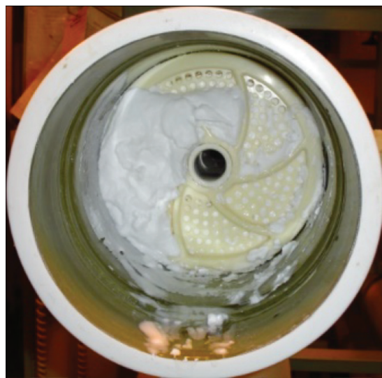
Figure 3 – Scaling on a membrane surface
