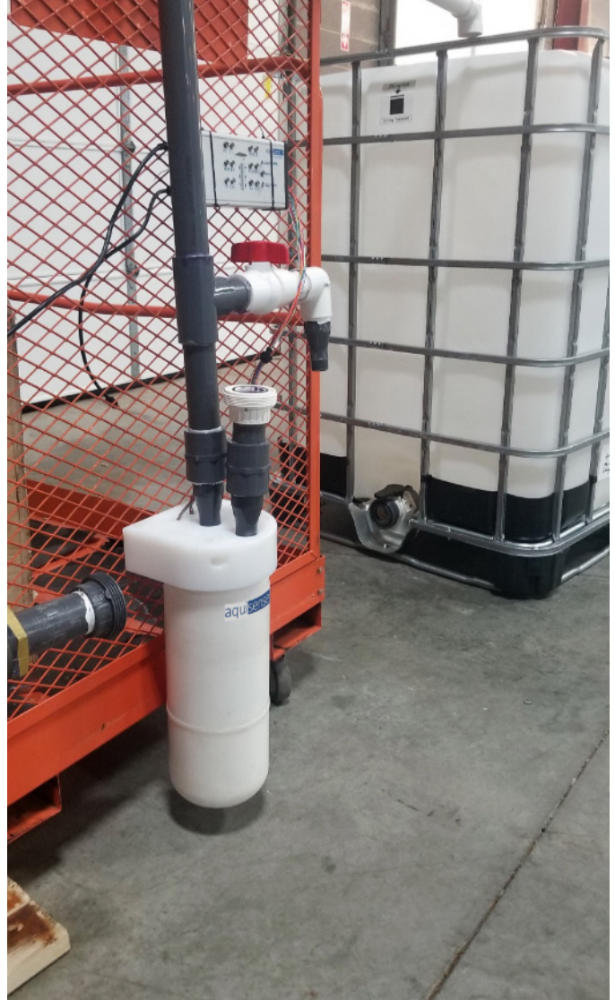
Figure 3. 20 gallons per minute UV-C LED Water Disinfection System Courtesy of AquiSense Technologies
