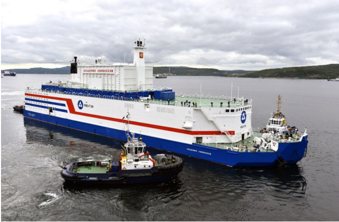
Figure 4. Ship-based nuclear generation for commercial power and heat. In 2020, the floating Russian nuclear power station Akademik Lomonosov moored in an arctic port completed commissioning and began supplying power to the Bilibino regional power system and heat to the port town of Pevek. Photographer: Lev Fedoseyev via Getty Images. Used with permission.
