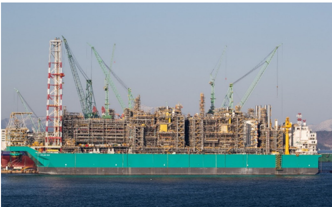
Figure 5. Ship-based production of fuels and other commodities. The petroleum industry has moved to floating production, storage, and offloading platforms (FPSOs). The Petronas Dua floating liquefied natural gas (LNG) vessel is pictured during construction at the Samsung Heavy Industries Co. shipyard in Geoje, South Korea in 2019. Photographer: SeongJoon Cho/Bloomberg via Getty Images. Used with permission.
