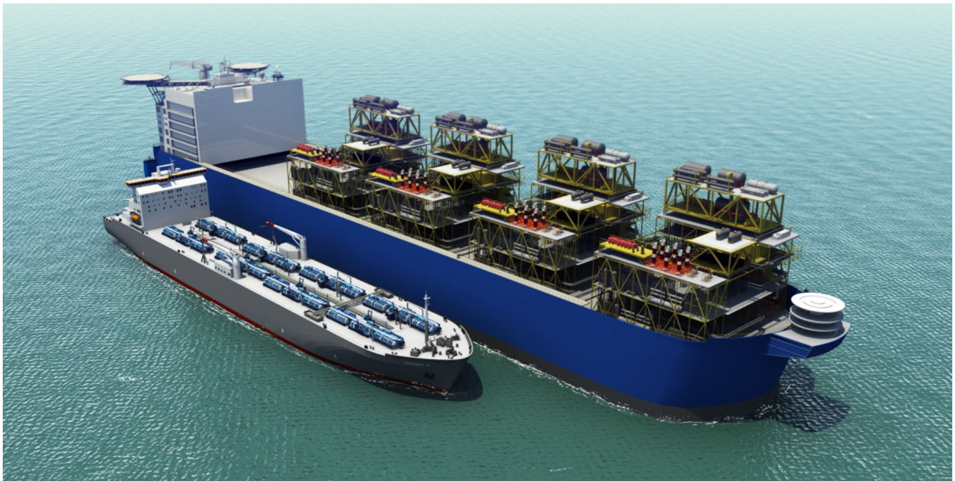
Figure 11. Scenario 1 – FPSO platform preparing to offload ammonia to tanker for delivery to point of use or subsequent distribution
