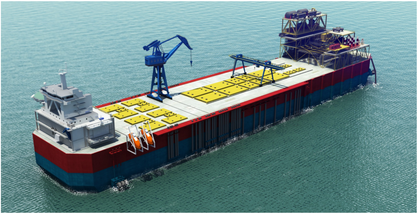
Figure 18. Scenario 3 — Power, ammonia, and desalination polygeneration via an FPSO moored close to shore for flexible product delivery to land. Not shown are pipelines and underwater transmission cables sending products to shore.
