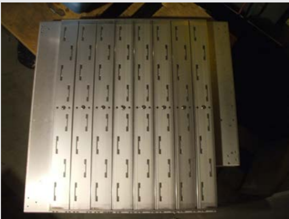
Figure 11. A typical “flat panel” millimeter wave base station antenna. Each small vertical element is an individual antenna. Courtesy of Bob Conley, Eigenwireless
