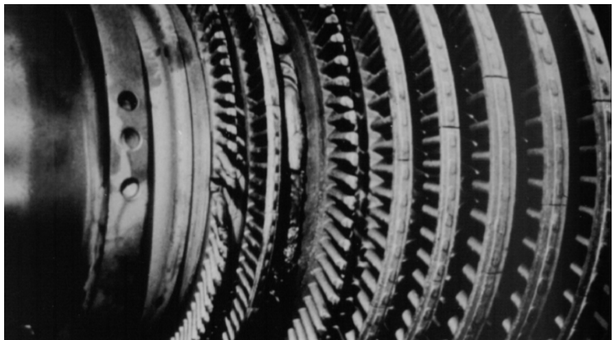
Figure 1 – First several rows of a turbine damaged by water induction
