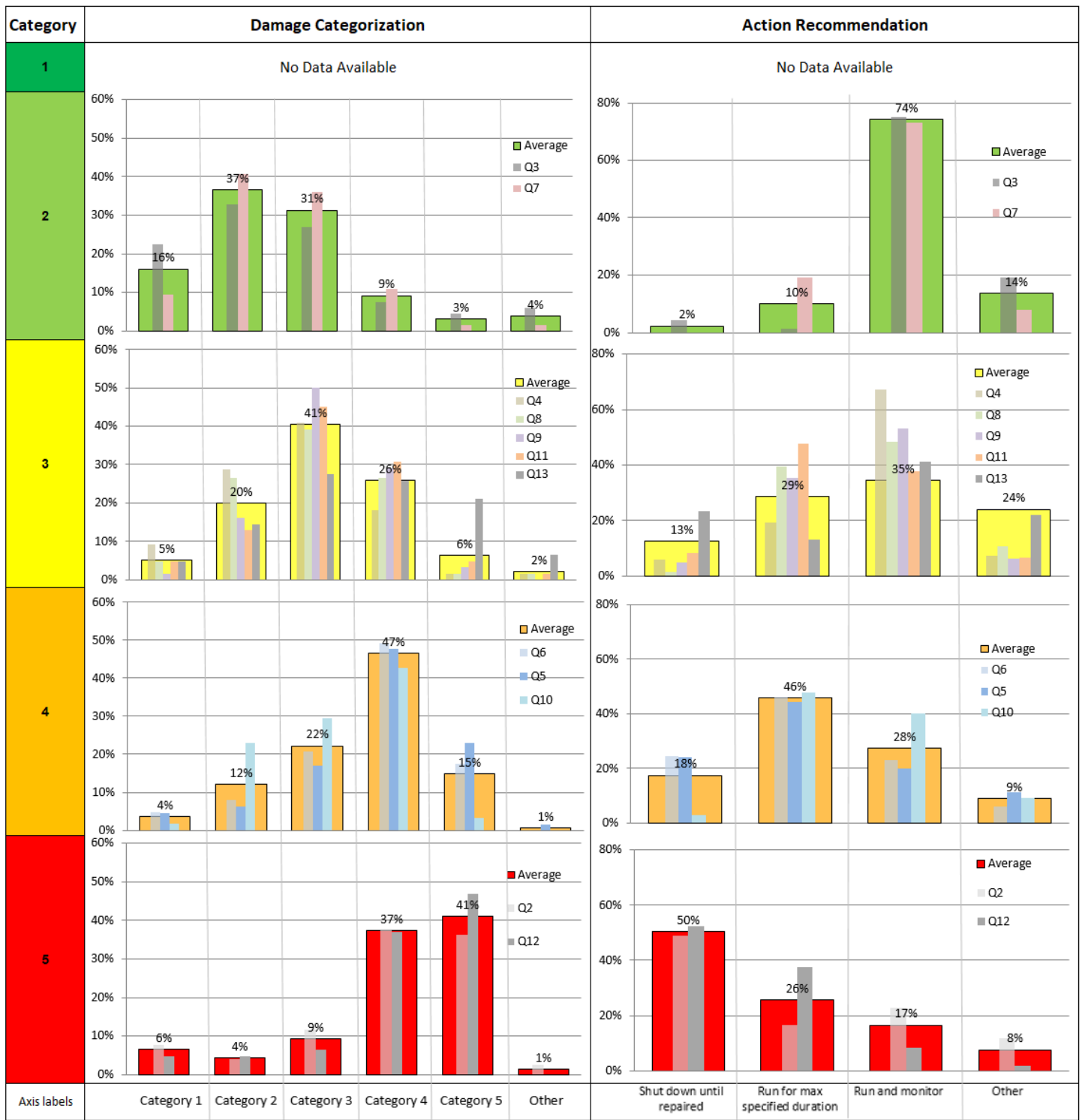
Figure 2-1 Damage categorization and action recommendation distributions. “Q” indicates question.
