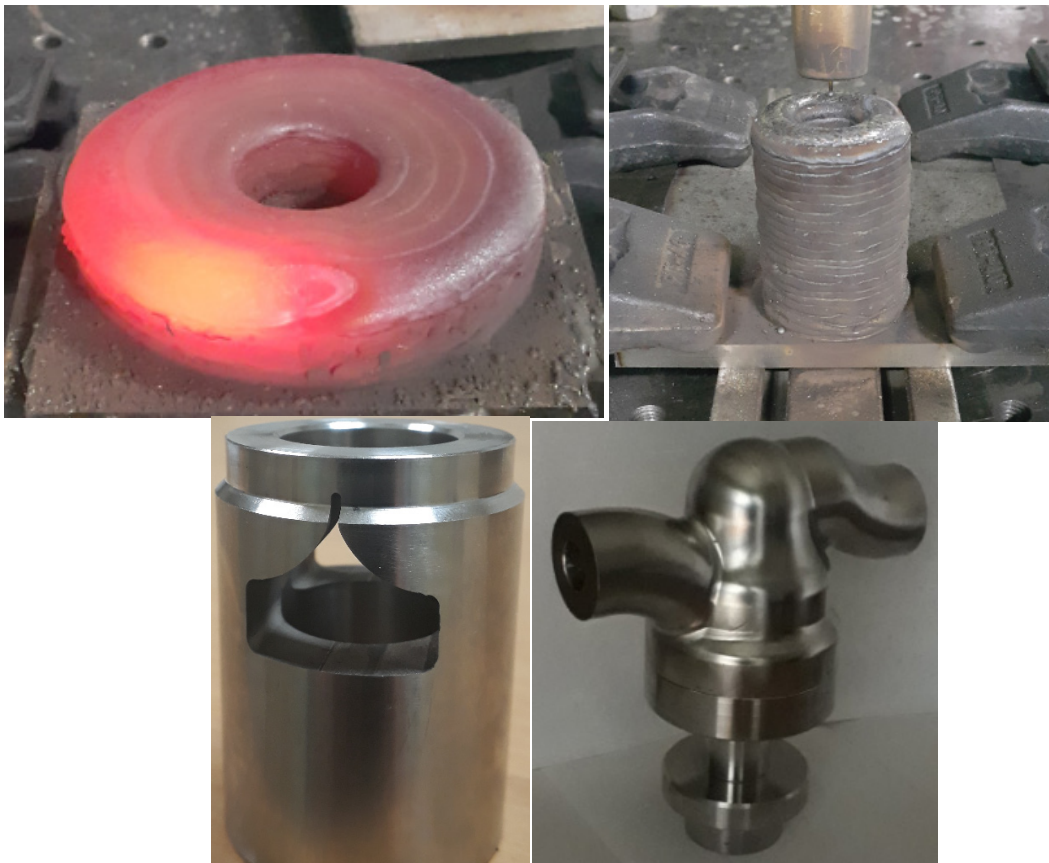
Figure 2. Valve cage in 316L stainless steel in process using GMA-DED, and cage and valve body after final machining Used with permission from Best Engineering in Energy Solutions
