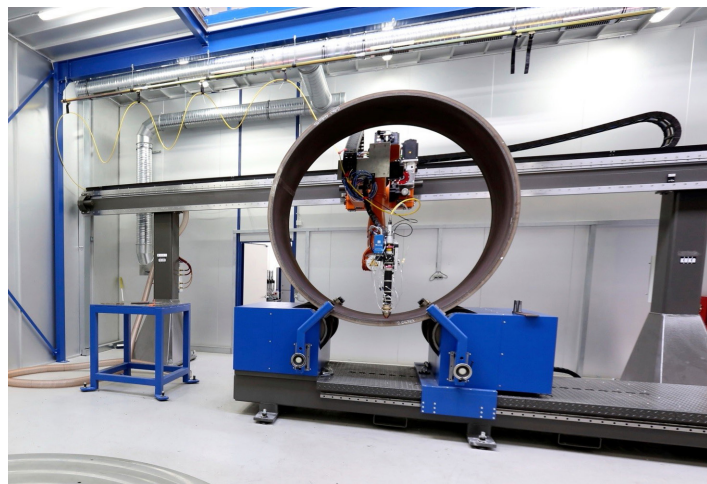
Figure 3. Fiber-coupled diode laser head mounted to robotic arm at the Nuclear Advanced Manufacturing Research Centre facility in preparation for ID cladding [2]
