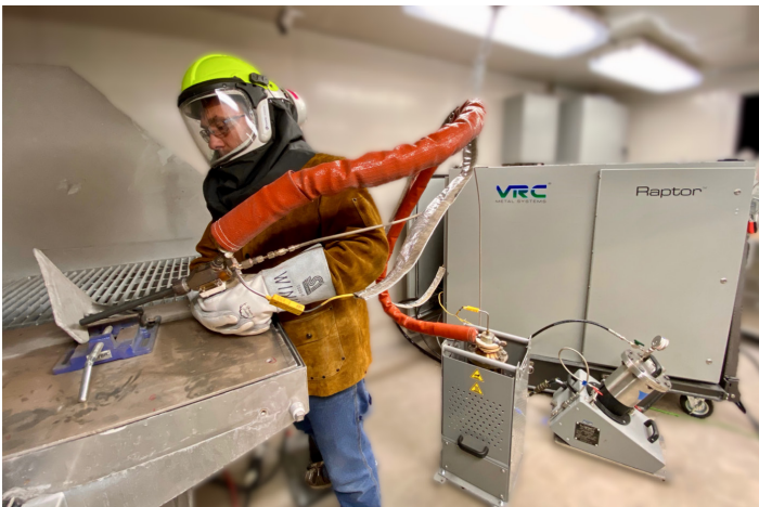
Figure 3. Example of a manual cold spray application Used with permission from VRC Metal Systems
