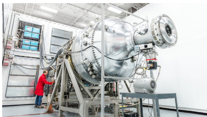
Figure 3. General Fusion’s latest generation of plasma injector (© 2018 General Fusion. Used with permission.)
