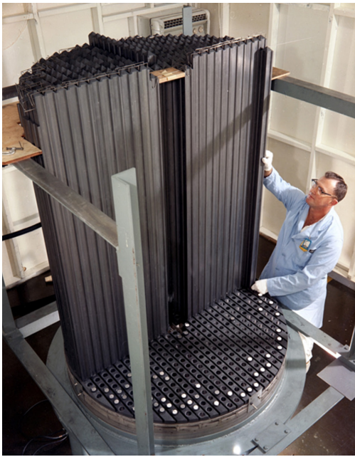
Figure 1. LEFT – Assembly of the core of the Molten-Salt Reactor Experiment, illustrating scale and configuration of core internals. RIGHT – View from above of MSRE reactor cell containing primary system. Pictured are the reactor vessel in upper center, heat exchanger in lower center, and fuel salt pump in left center of image. Scale indicated by worker on top of reactor vessel [Source: Oak Ridge National Laboratory for the U.S. Atomic Energy Commission, ca. 1964.]
