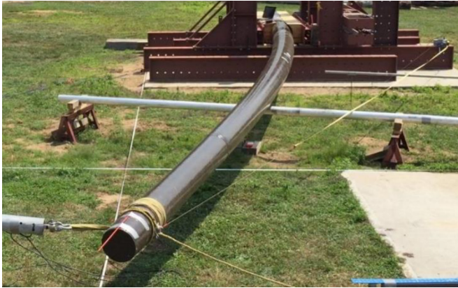
Composite Pole Undergoing Testing to Failure
