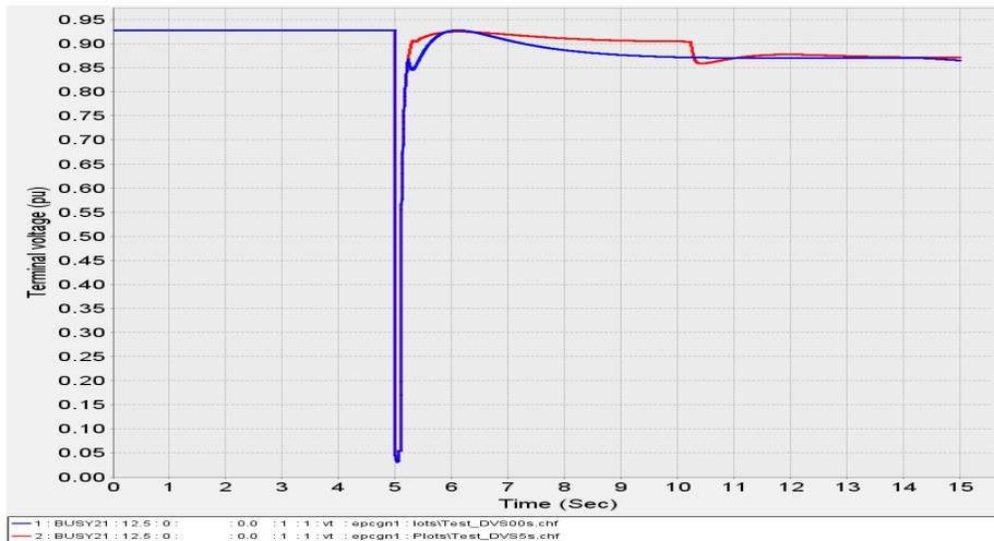
Figure 2-6: Voltage magnitude for two different values of Tdb (Blue - Tdb = 0.0s, Red - Tdb = 5.0s)
