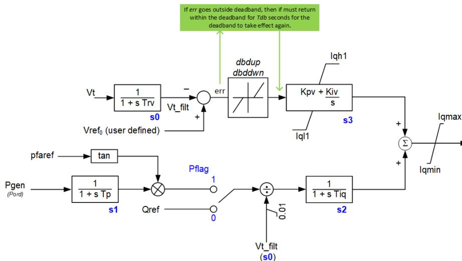
Figure 2-2: Proposed voltage control loop
