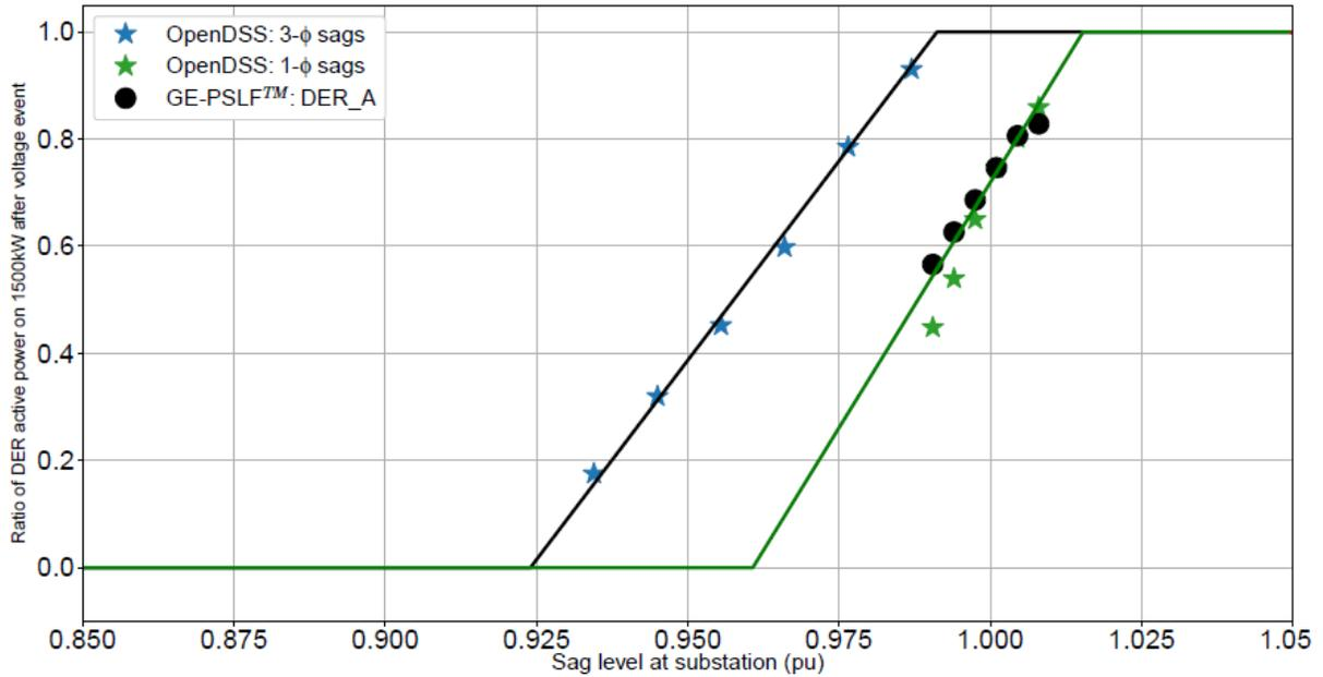
**Figure 3-2: Representation of second partial trip characteristic in DER\_A model to approximate tripping of DER to unbalanced faults**
