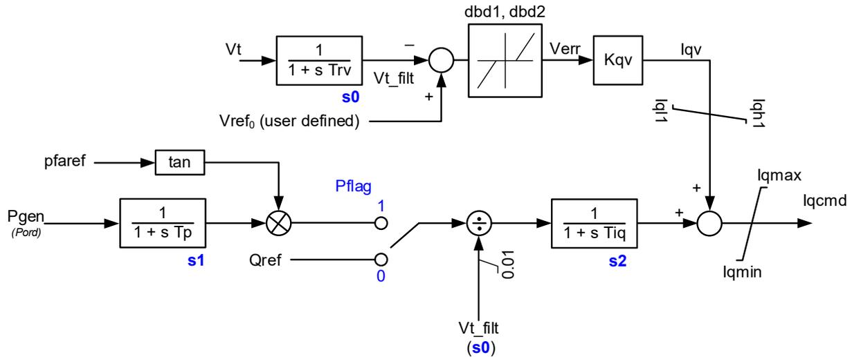
Figure 2-1: DER\_A voltage control loop
