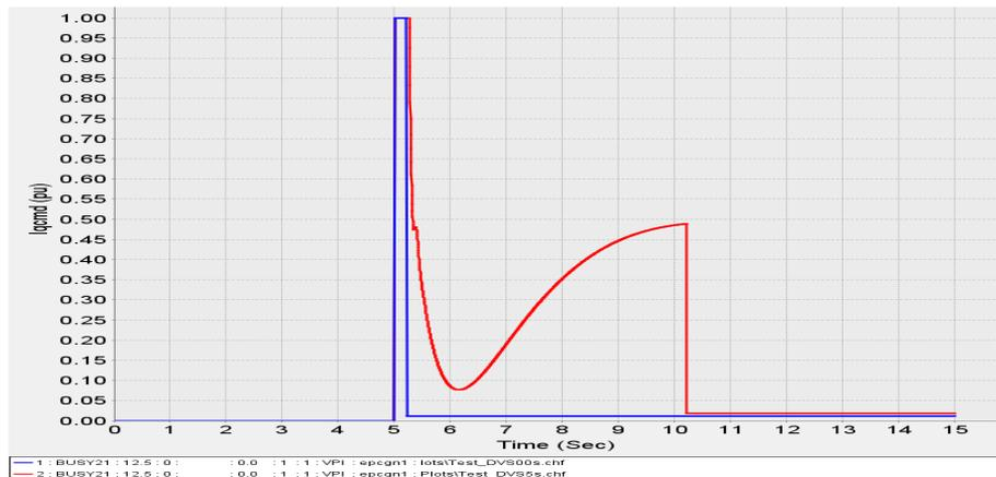
Figure 2-7: Reactive current command for two different values of Tdb (Blue - Tdb = 0.0s, Red - Tdb = 5.0s)
