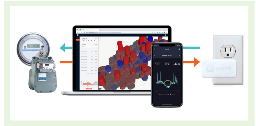
Wireless hardware deployed at the meter and inside buildings supplies real-time usage data to support analysis, visualization, and informed interventions by customers and utilities.
