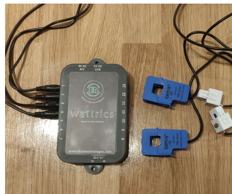
Wattrics devices, which apply current transducer clamps to monitor up to 14 circuits (left), were installed in one of the main electrical cabinets in a community building (right), as well as in five residential units.
