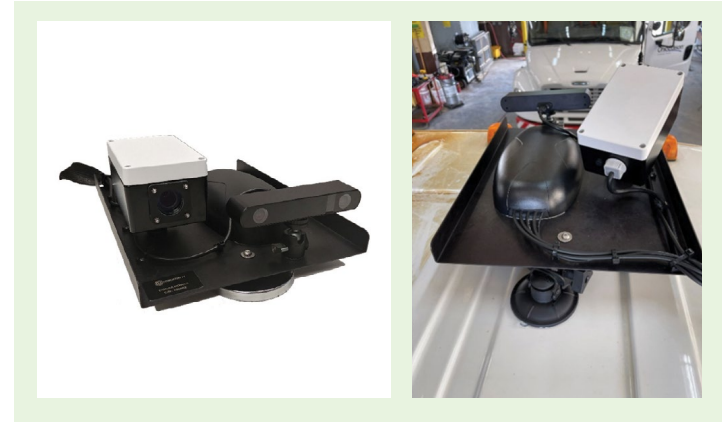
The Inspector Edge's exterior unit features rooftop-mounted cameras for capturing images of roadside distribution infrastructure.
