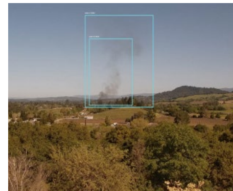
Pano AI stations deployed on existing towers (left) deliver live-feed images that are analyzed for smoke detection (right) and wildfire risk assessment.
