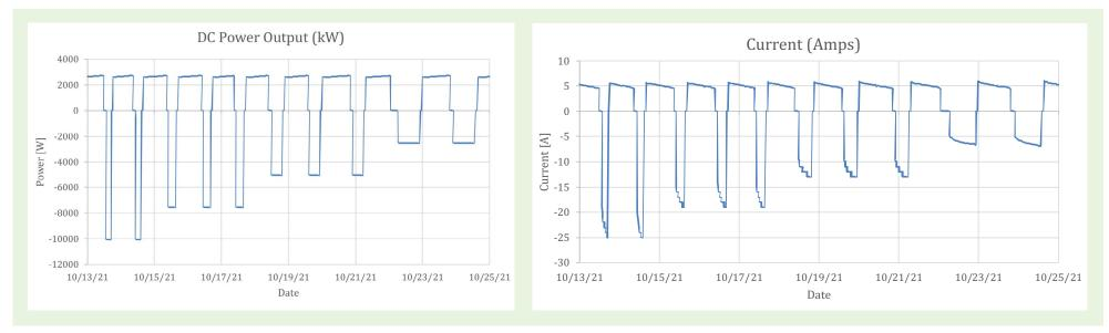
Sample energy capacity testing results show power (left) and current (right) levels through 12 charge/discharge cycles performed at various rates. Discharge periods ranging from 4 to 16 hours demonstrate the UEP storage system's applicability for long-duration use cases.
