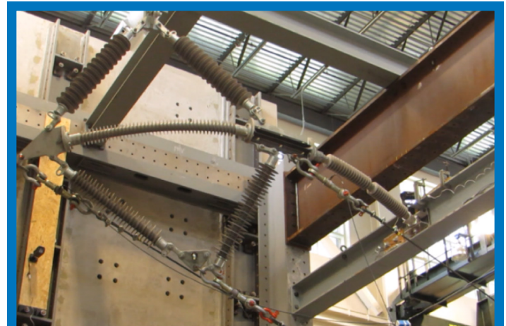
Figure 21: Mechanical testing of 115kV compact assembly [Courtesy of National Grid USA]
